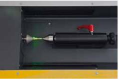
The accuracy of measurement of the dimensions of the inserts and ferrules are essential for the proper use and operation of the QUADRA System. The measuring device we added to pursue this improvement in accuracy is a laser-scanner. With this equipment you get accurate and precise measurements of the fittings.
