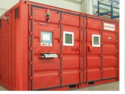
Proof pressure test stand able to pressurize hose assemblies up to 6.000 bar (87000 psi)
