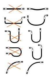
Since hose may change in length under the surge of high pressure, provide sufficient slack for expansion and contraction.
