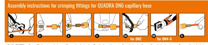
Cut the QUADRA capillary hose to the required lenght using the special WXAOO4 cutter Slip the nut over the hose (depending on fitting type). Ensure that the threaded side is pointing towards the end of the hose that needs the assembling.
