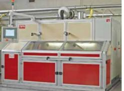
Burst test stand capable of performing burst tests on hose assemblies up to 10.000 (145000 psi)
